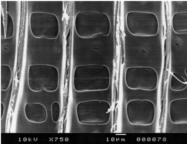
**Fig. 4.** Radial section of acetylated pine wood (WPG between 16% and 18%). Window pits with undamaged membranes
