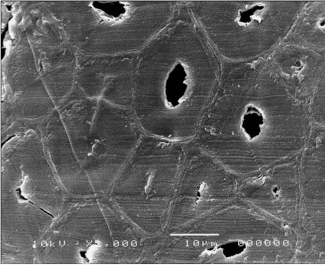
**Fig. 1.** Acetylated beech (WPG between 18% and 20%). Cross-sectional view of swollen fibre tissue. Some lumina are completely closed
