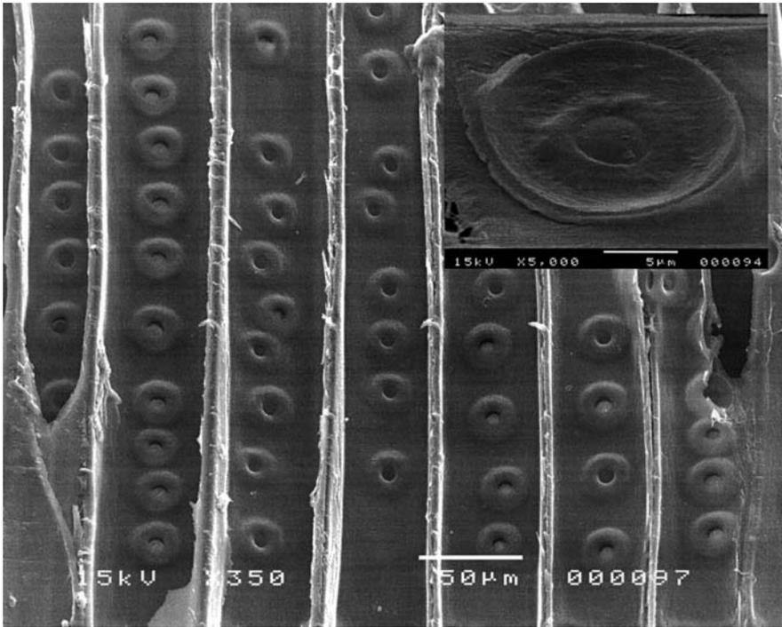
**Fig. 3.** Radial section of acetylated Norway spruce (WPG 16%). Bordered pits are undamaged. *Window:* opened bordered pit chamber with intact torus and margo
