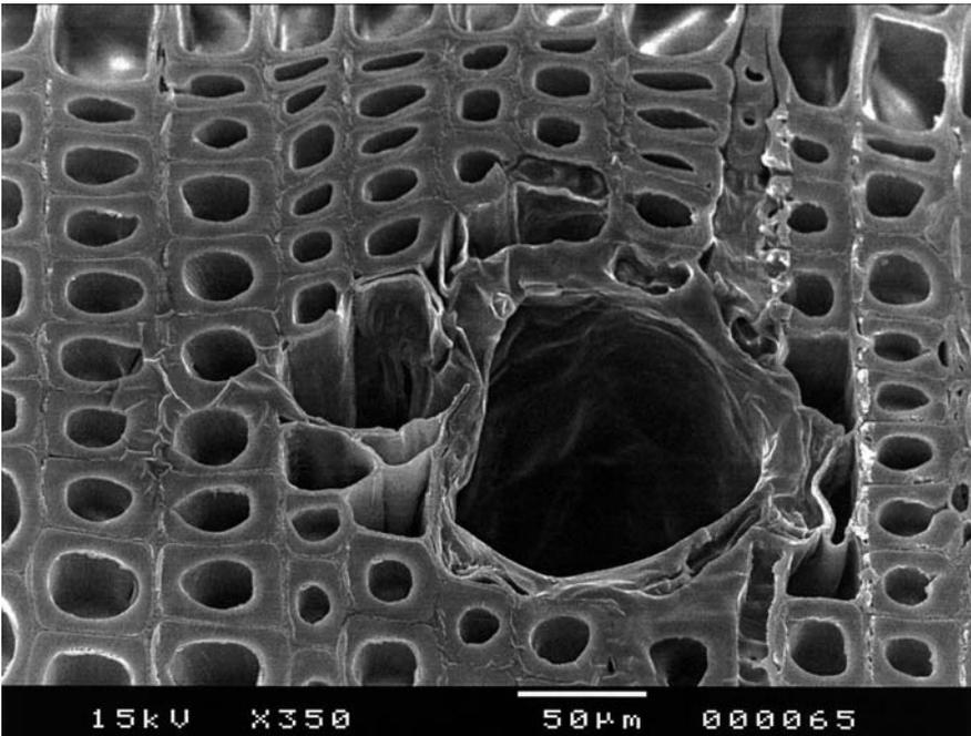
**Fig. 2.** Acetylated Scots pine (WPG between 16% and 18%). Cross-sectional view of latewood with a resin canal. Epithelia cells are untouched and partly filled with resin
