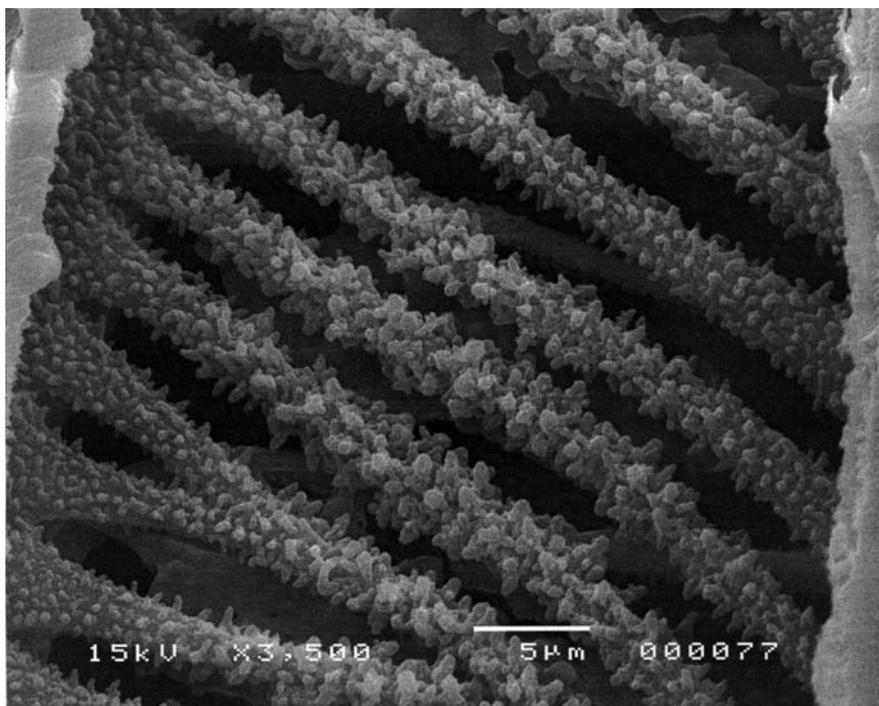
**Fig. 5.** Longitudinal section of acetylated beech wood (WPG between 18% and 20%). Scalariform vessel perforation with vestures, unaffected by the treatment
