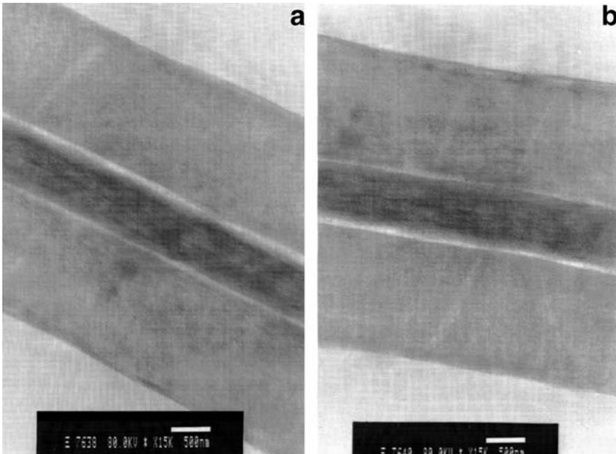
Fig. 6a, b. TEM-micrographs of a non-treated (a) and an acetylated (b) tracheid cell wall of the same tree ring. The WPG of the acetylated sample was 17%. The stronger lignified areas appear darker due to permanganate contrast. *ML*, middle lamella; *S2*, secondary wall 2
